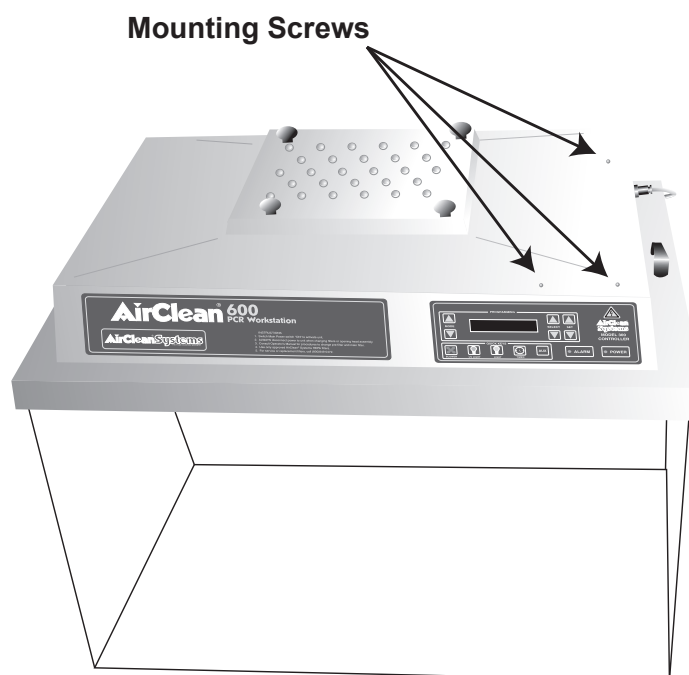
Figure 9, Removing the UVTest™ Controller from the AC632 model.
